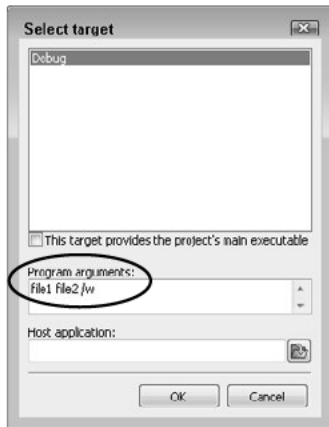
Figure 18-9: You can set up the project to pass arguments to the program when executed from Code::Blocks.
