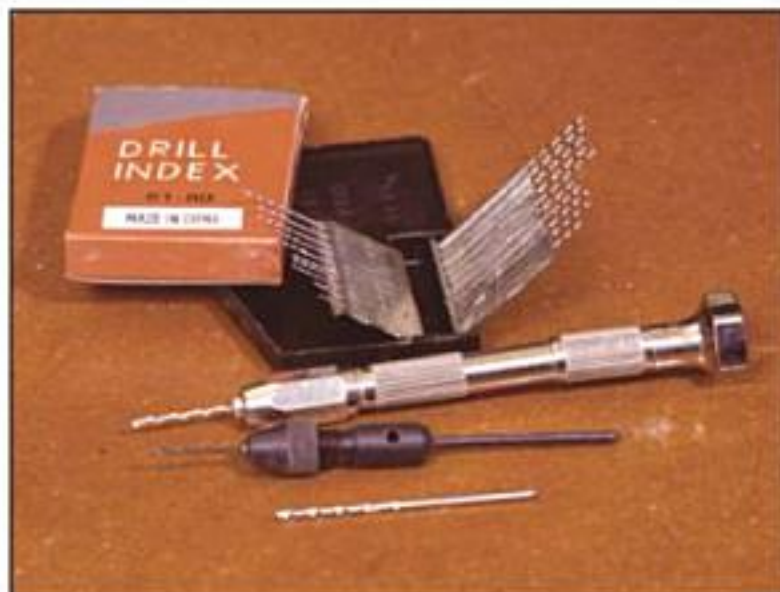
A 1/16" drill bit is shown on the bottom, for size comparison. This hand vise works well on thin woods. The complete set of pin drills are shown in its box.
