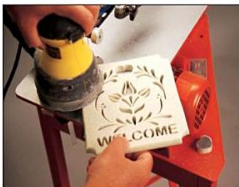
Out of orbit: Orbital sanders, like this one, produce a smoother finish on Corian because they create random sanding strokes.
