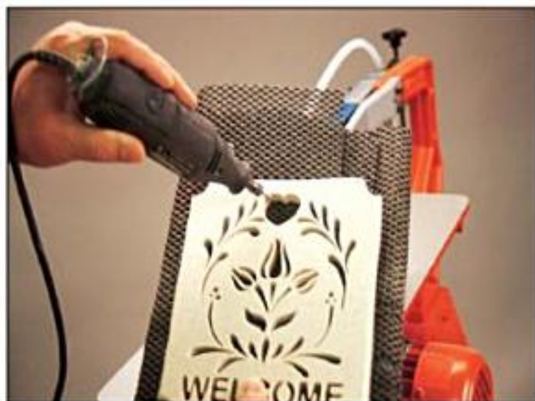
A "kinder-gentler" tearout: Saw marks can be dressed with a rotary polishing tool or removed with sandpaper and a dowel.
