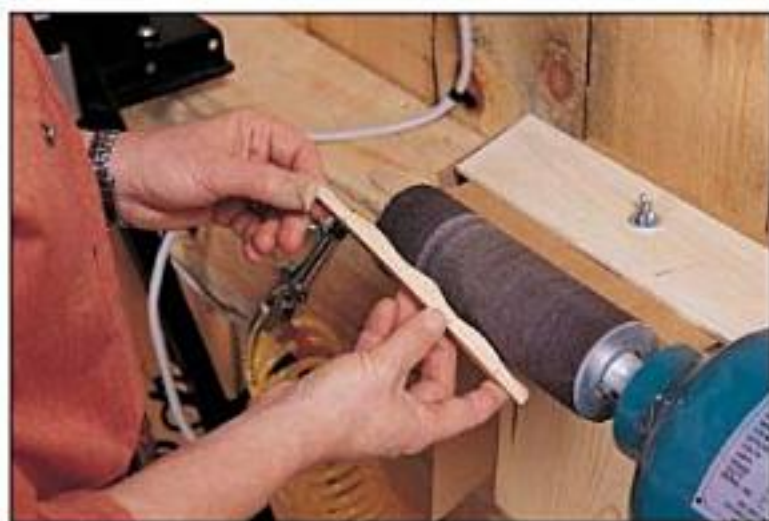
Step 13: The basket's dips can be contoured using a 2½", or smaller, drum on a flexible drum sander. However, the dips can be carved or scrolled too.
