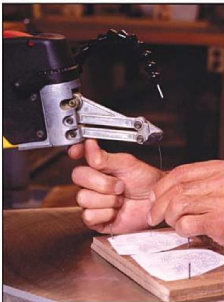
On the Dewalt, you can feed the blade in from the top, while the work is lying on the table.
