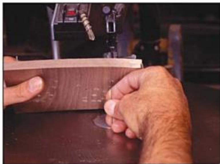
On most saws, like the Delta Q3, you feed the blade in from the bottom.
