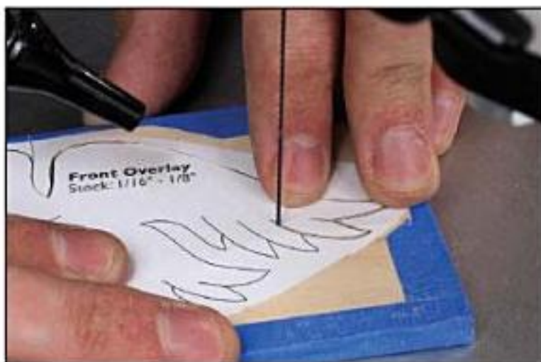
Veining can give your projects a lifelike appearance. Many times veining areas will be as simple as cutting inward from the outside edge.
