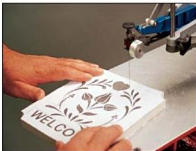
Fun with floral frets: When sawing the ornate parts of the floral pattern, scroll the larger sections first, then the smaller pieces.
