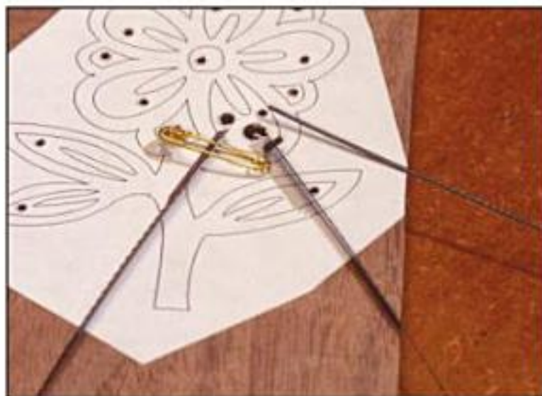
The type of blade you use will have a lot of bearing on the size of the blade entry hole. The blade on the right is a # 2 blade, and it requires a 1/16" hole. The blade in the middle is a regular pin-end blade. It needs a 1/32" hole. The blade on the left has had its pin removed. With the pin out of the way, we can go down to a 1/64" hole.
