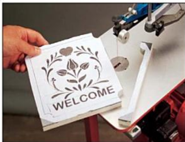
On the edge: When scrolling the Floral Welcome Trivet, make the outside cuts first. Take your time and use a steady feed rate.
