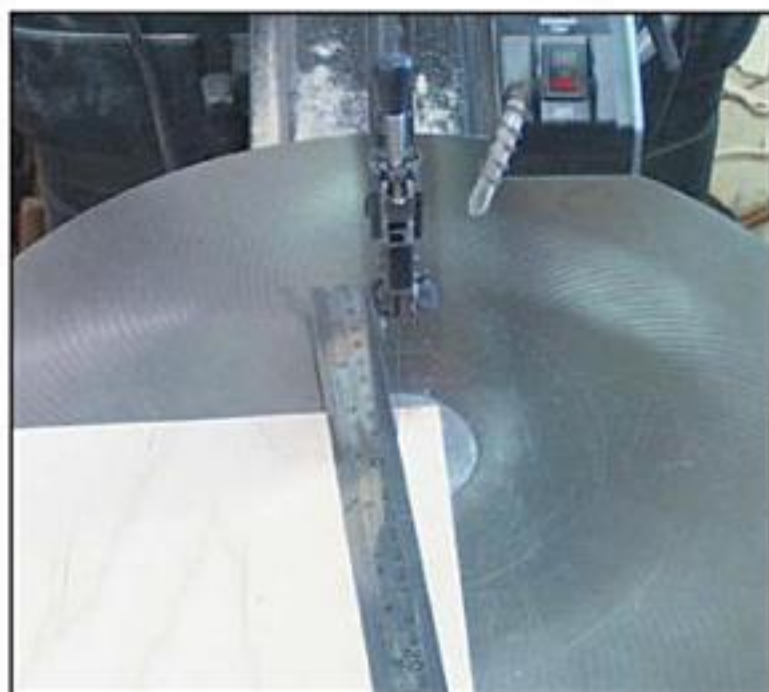
With a ruler lying on the line, we really see how far off the blade is cutting.
