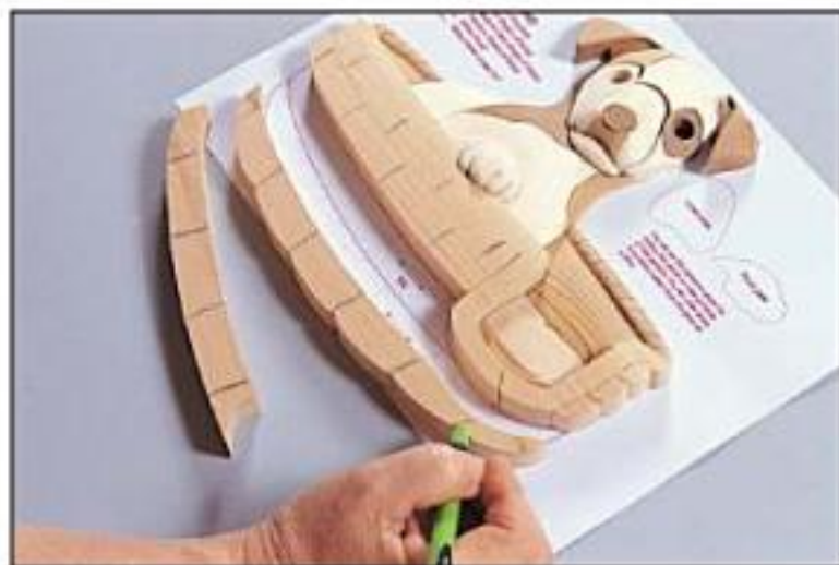
Step 12: The dashed dips in the basket section of the pattern create an alternating weave effect.
