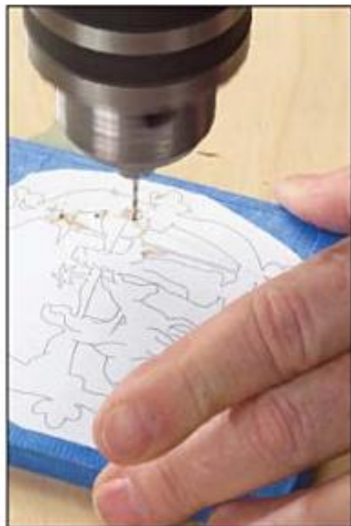
A drill press is recommended for perpendicular entry holes.
