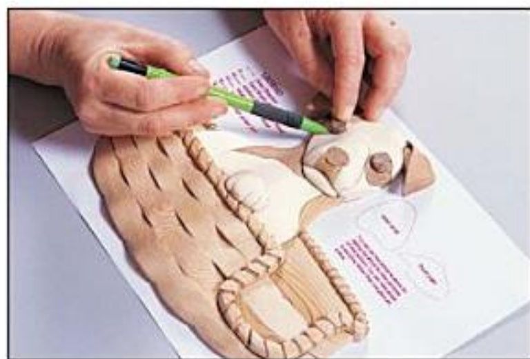
Step 15: Sand the eyes slightly below the pencil line because the eyes will be a little thinner than the area around them.
