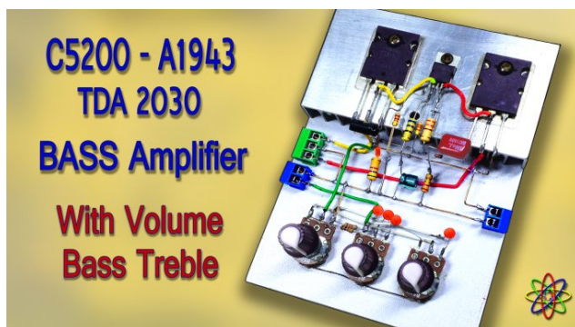
Heavy Bass Powerful Amplifier of c5200 A1943 & TDA2030 with Volume Bass Treble – DIY Homemade class A
