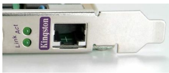
Figure 1.24 – RJ45 Female End
