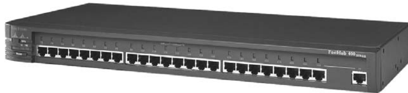
Figure 2-23 Hubs Have Several Ports
