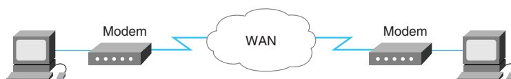
FIGURE 9-7 A WAN can handle analog and digital signals through a modem connection.
