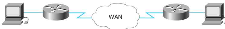
FIGURE 9-14 A typical point-to-point link operates through a WAN to a router, and to end systems on both ends of the link.
