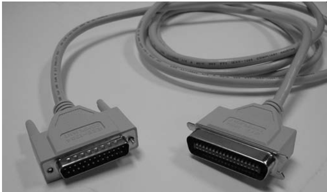
FIGURE 1.63 A typical parallel cable
