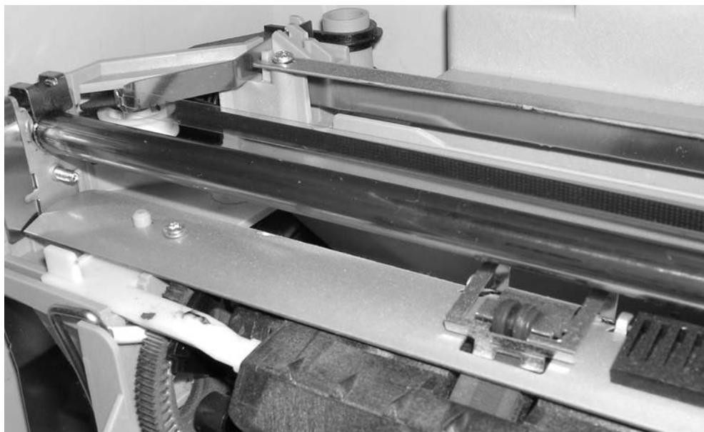
FIGURE 7.6 Stabilizer bar, carriage belt, and pulleys in a bubble-jet printer
