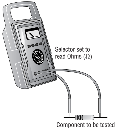
FIGURE 2.11 Connecting a multi-meter to measure resistance
