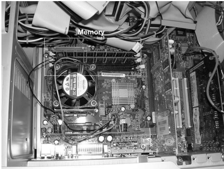
FIGURE 1.25 Location of memory within a system
