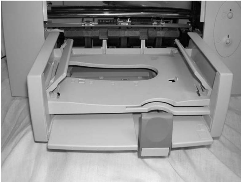
FIGURE 7.9 A paper tray on a bubble-jet printer
