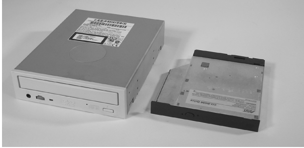
FIGURE 3.7 A desktop CD-ROM drive compared to a laptop CD-ROM drive
