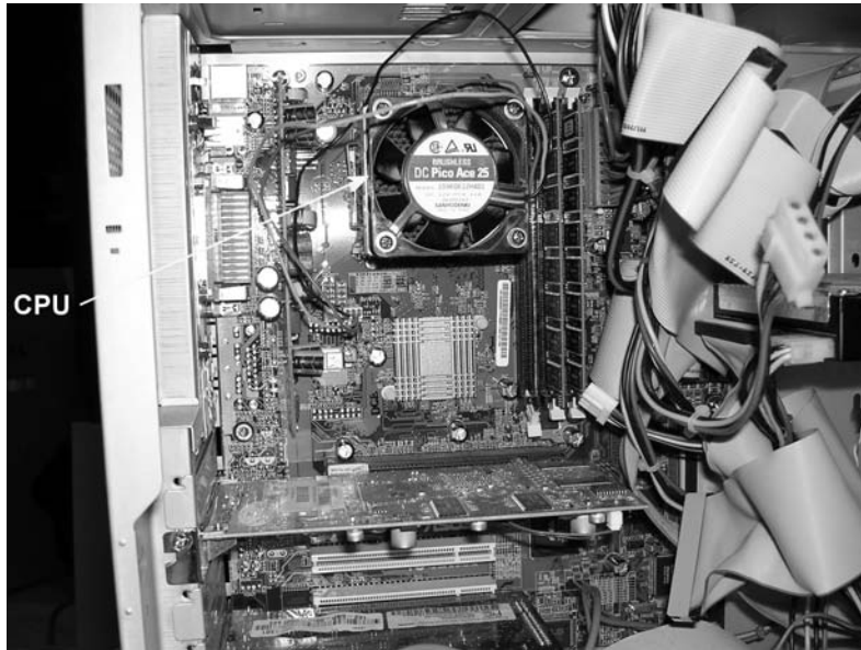
FIGURE 1.24 The location of a CPU inside a typical computer
