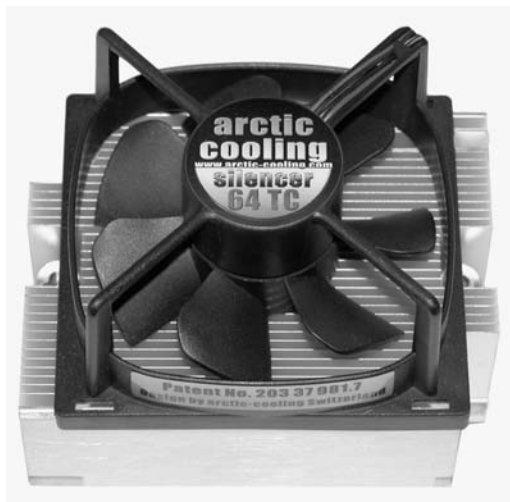
FIGURE 1.73 An active hard disk cooler
