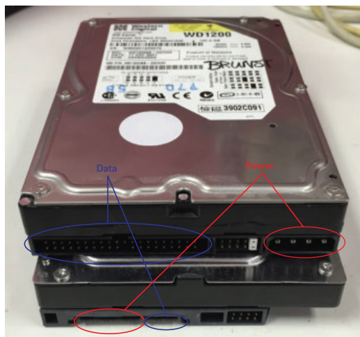
FIGURE 1.21 PATA/IDE and SATA hard drives
