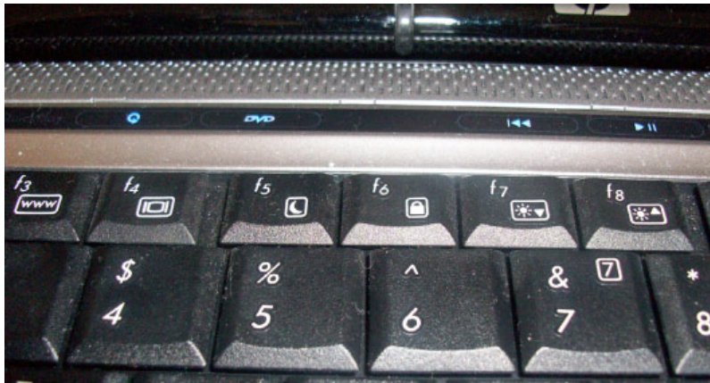
FIGURE 2.11 Video adjustment keys including F4 (LCD toggle), F7 (dim), and F8 (brighten)
