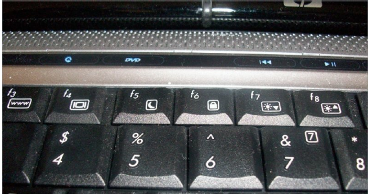
Figure 9.9 Video adjustment keys F4 (LCD toggle), F7 (dim), and F8 (brighten)
