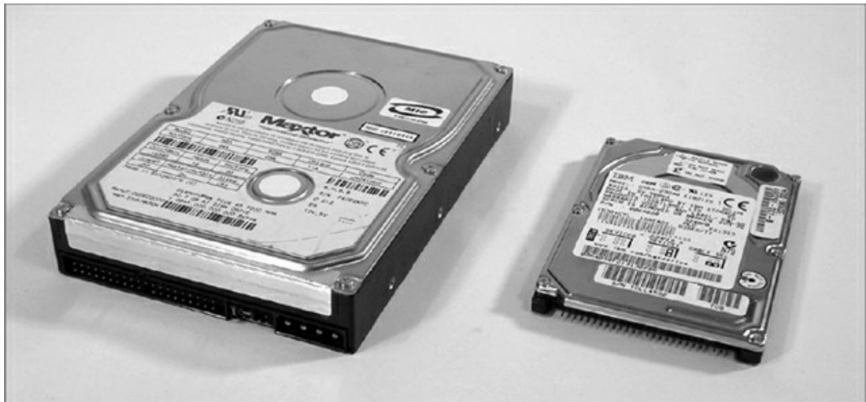
Figure 9.5 A desktop hard drive (left) compared to a laptop hard drive (right)
