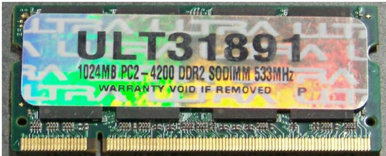
Figure 1.29 200-pin DDR2 SODIMM
