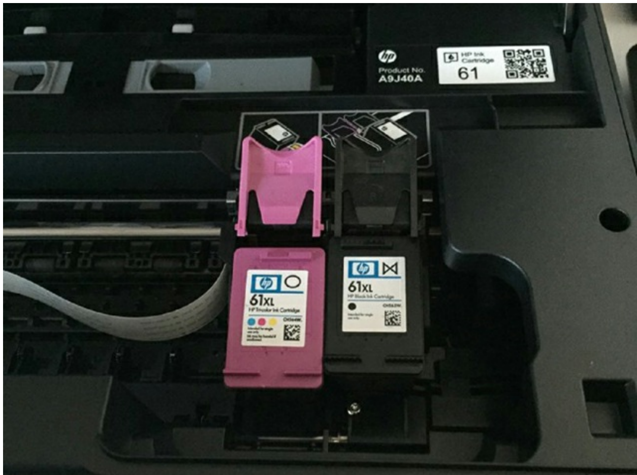
Figure 11.3 A print head carriage (holding two ink cartridges) in an inkjet printer
