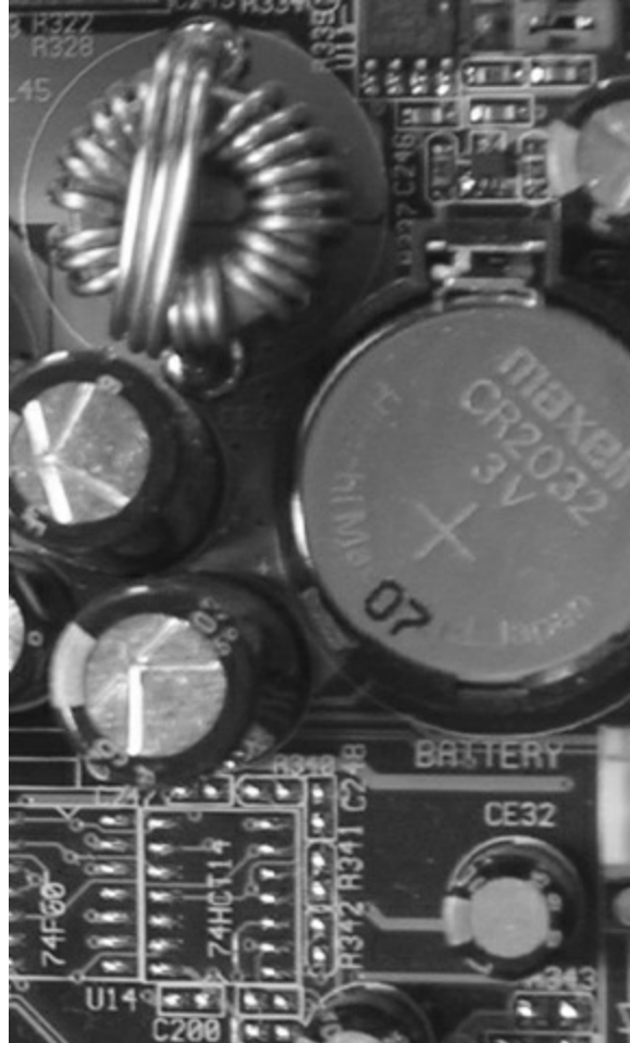
Figure 1.14 A CR2032 CMOS battery
