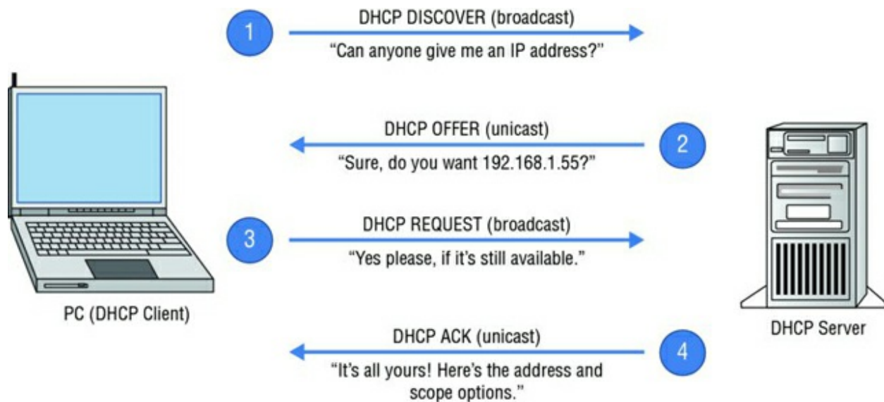
Figure 20.5 The DHCP request process
