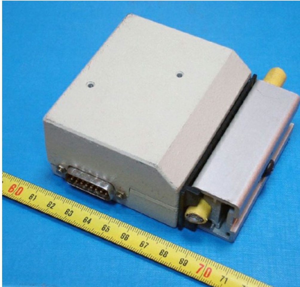
Figure 6.13 Thicknet transceiver and cable inside a vampire tap
