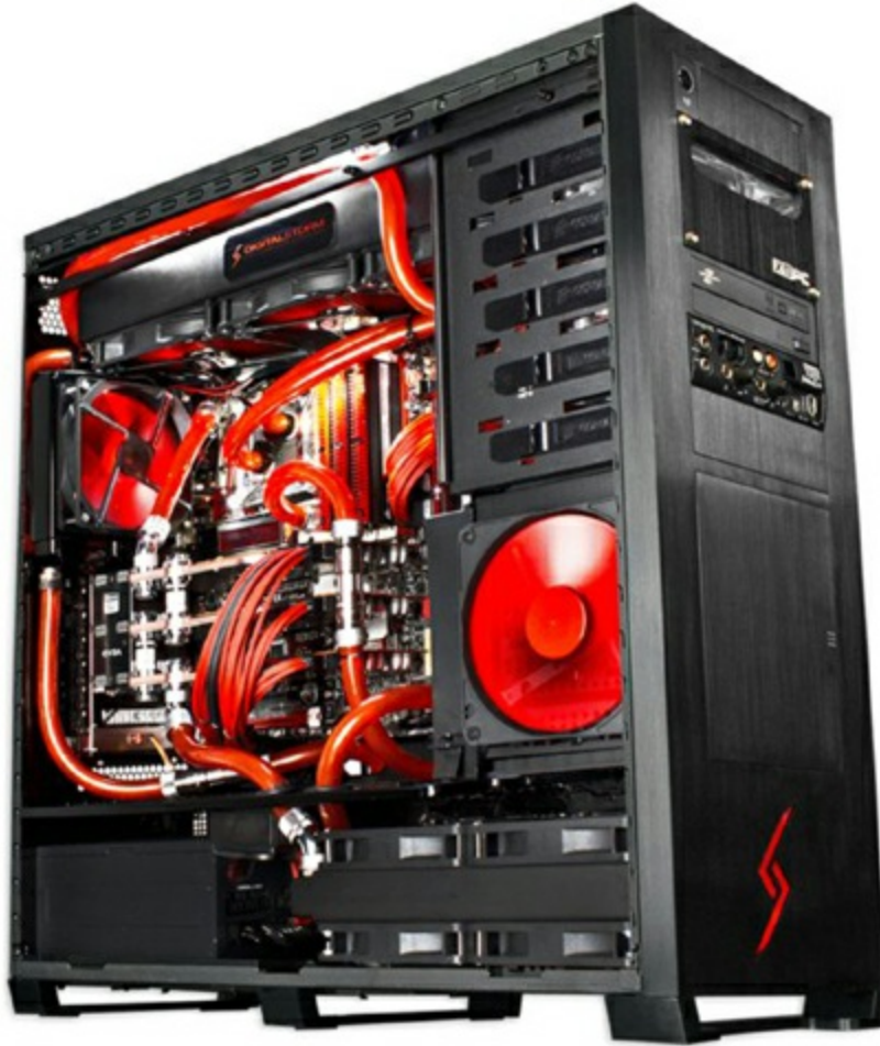
Figure 5.1 Gaming system with liquid cooling
