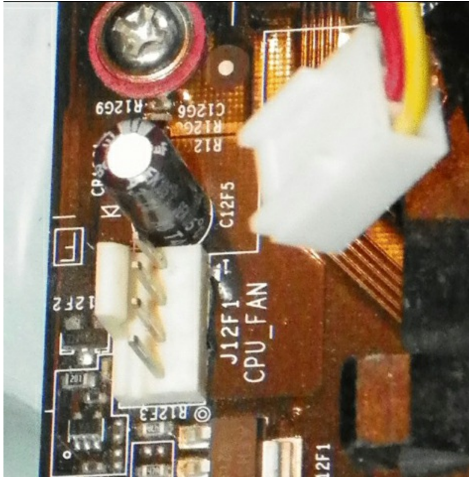
Figure 1.31 A four-pin CPU fan header
