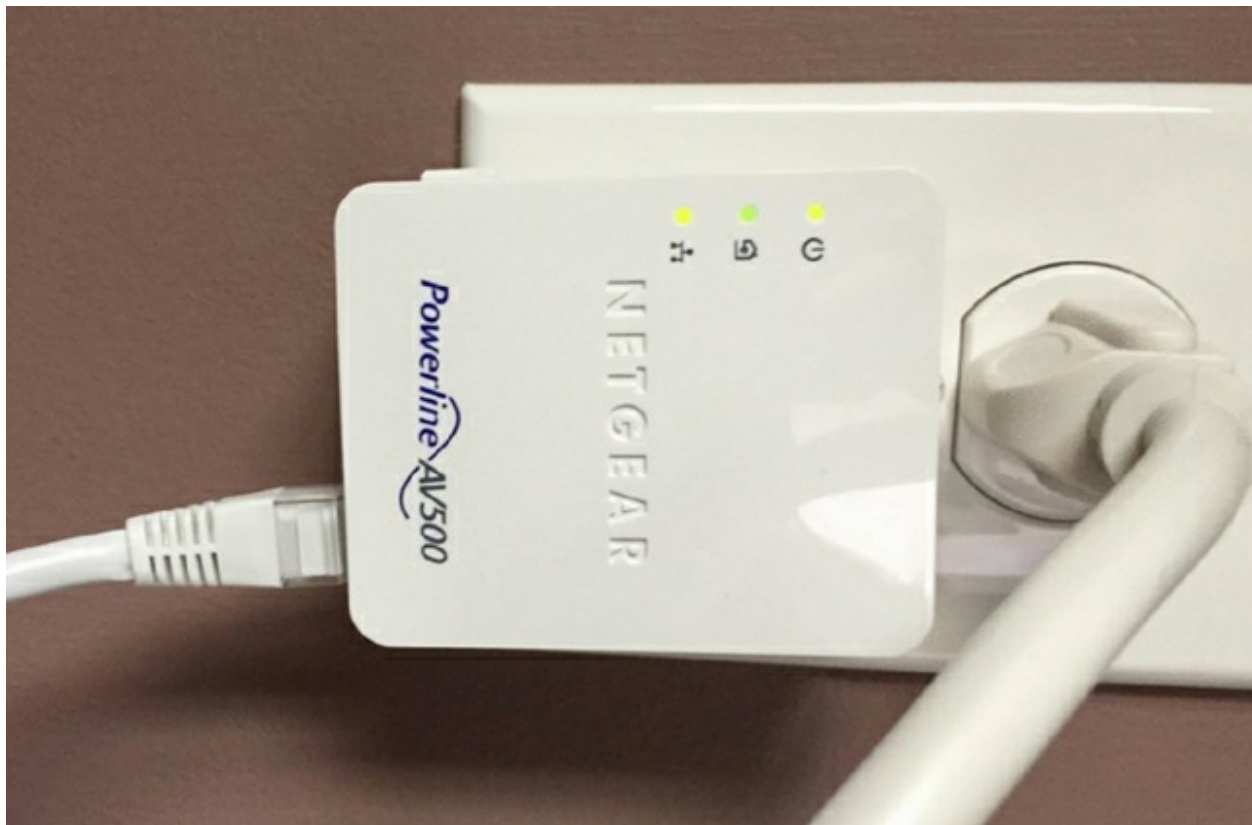
Figure 6.27 Ethernet over power adapter
