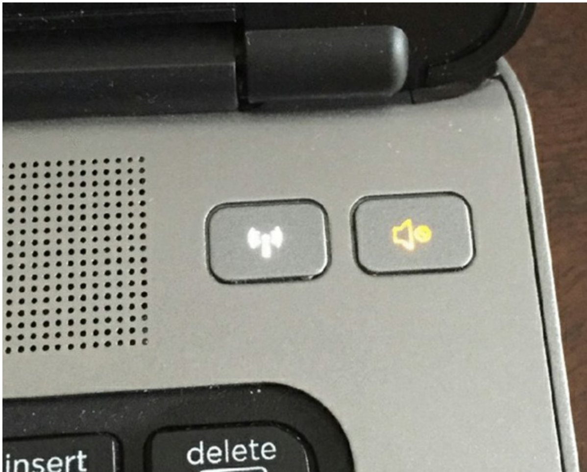
Figure 12.8 Network card toggle switch above the keyboard
