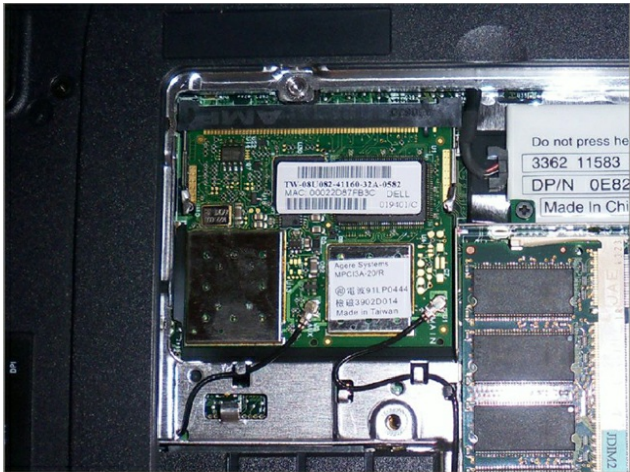
Figure 9.36 Mini PCI card installed in a laptop
