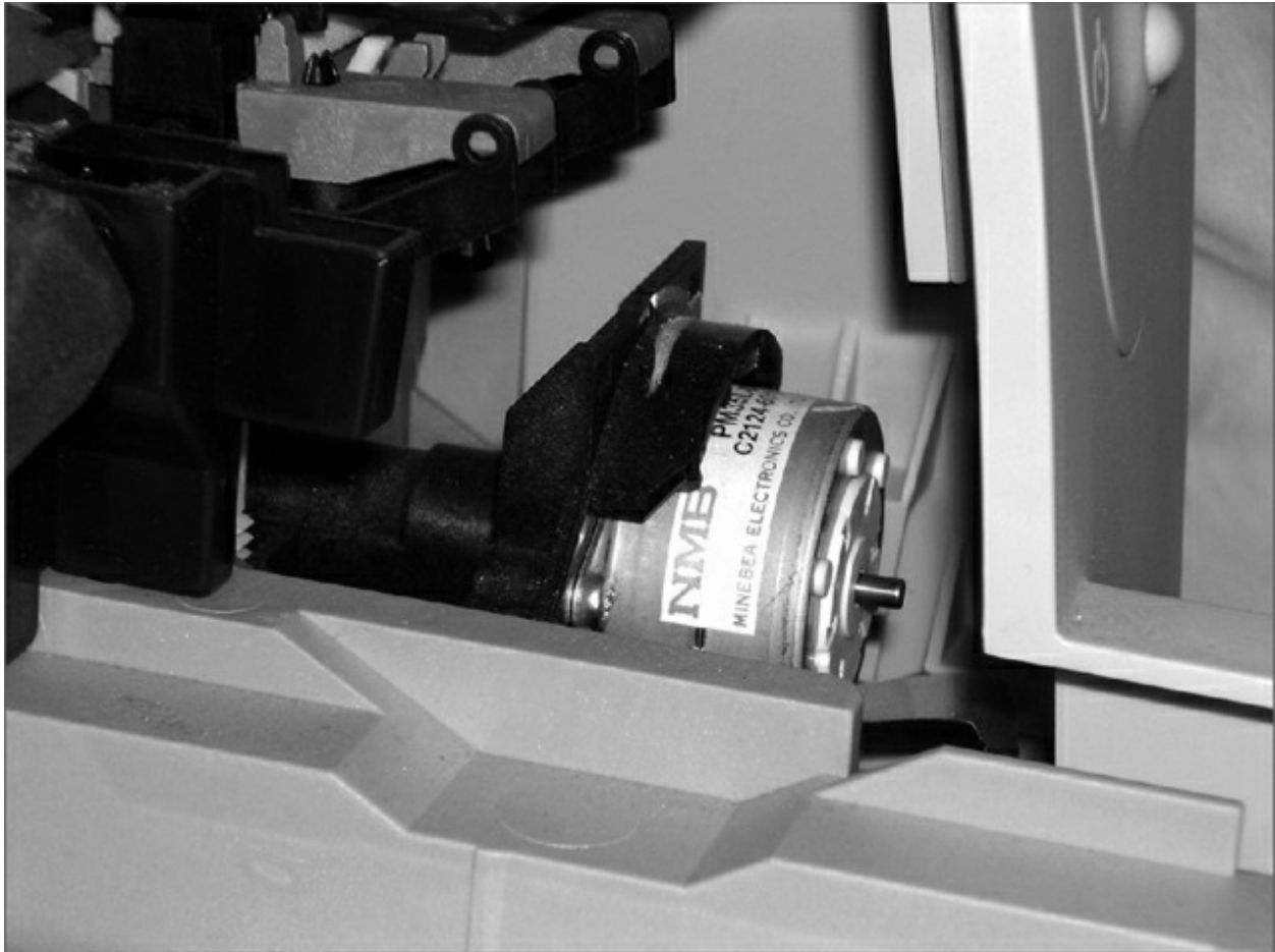
Figure 11.4 A carriage stepper motor
