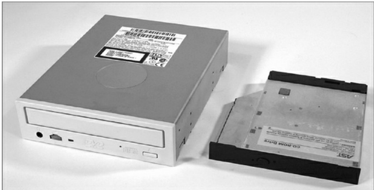
Figure 9.7 A desktop DVD drive (left) compared to a laptop CD drive (right)
