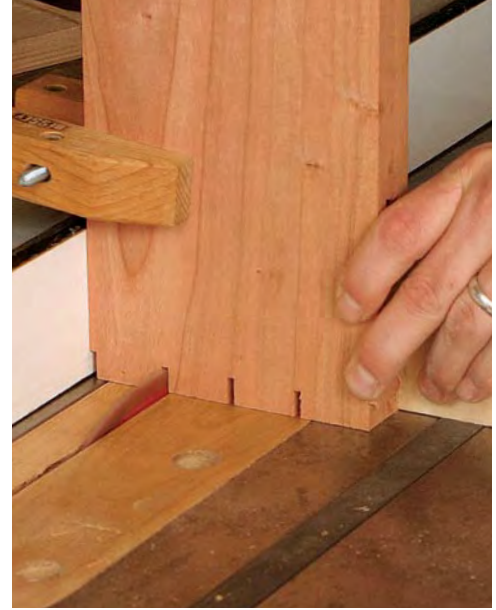
Lay out the tail centerlines. A single line is all that's needed to mark the tail centerlines (above). On the tablesaw, use the miter gauge with a tall auxiliary fence to make a sawcut at each centerline (right).
