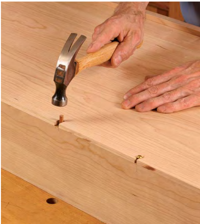
Center a dowel on the drawer bottom. The author measures for the center to lock in the location and uses a doweling jig to drill straight.
