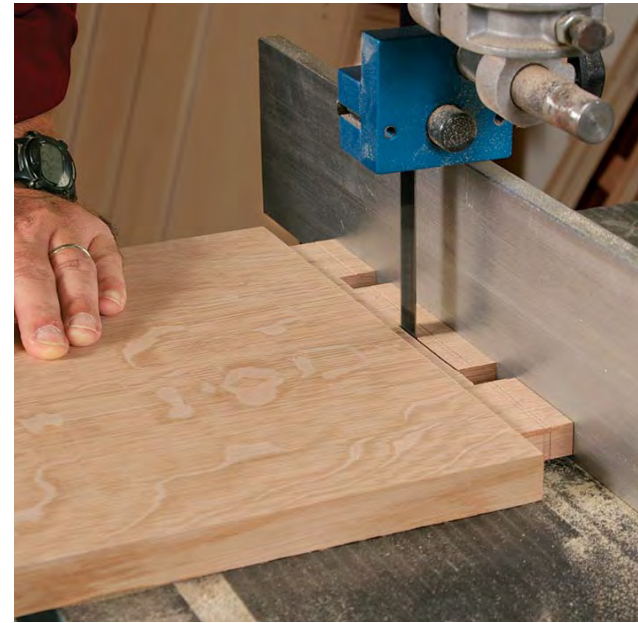
Saw off the stub tenon. Use the bandsaw to cut the stub tenons to length. The fence ensures a parallel cut.
