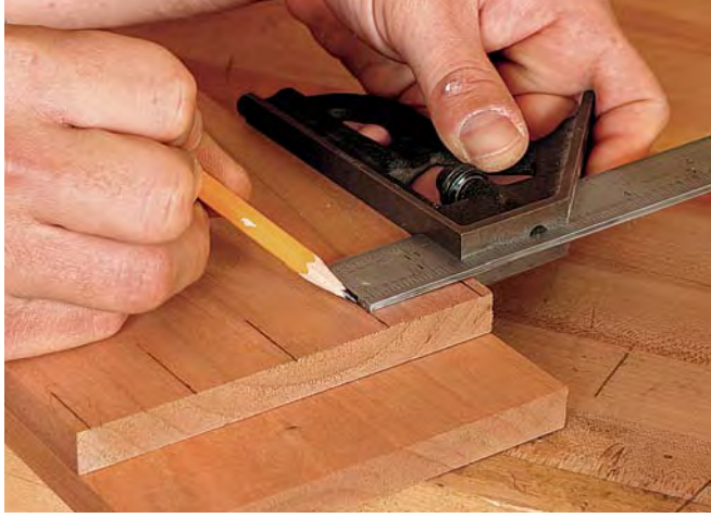
Lay out the tail centerlines. A single line is all that's needed to mark the tail centerlines (above). On the tablesaw, use the miter gauge with a tall auxiliary fence to make a sawcut at each centerline (right).
