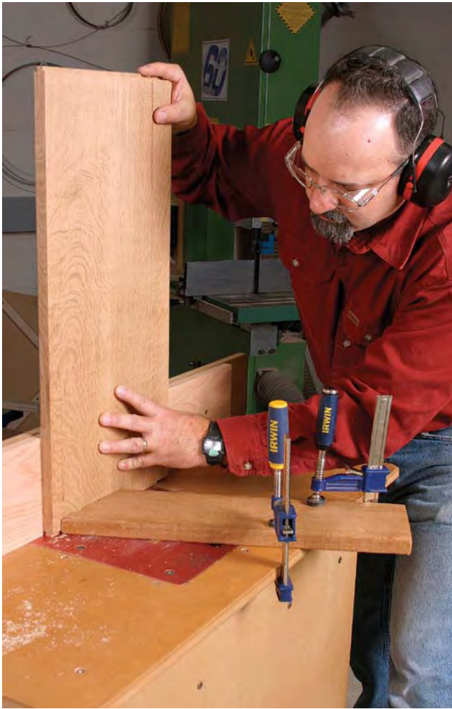
Vertical dividers. After cutting the dividers to length, use the dovetail bit to cut the keys. A tall fence supports the long boards and a featherboard keeps the piece snug against the fence.
