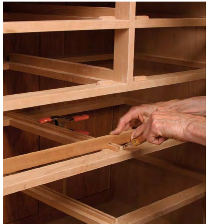
Use a stick to keep it on track. To keep the guide centered as you mark around it, use a notched stick at the front and then the back. Glue and screw the guide only to the front and back rails of the web frames.
