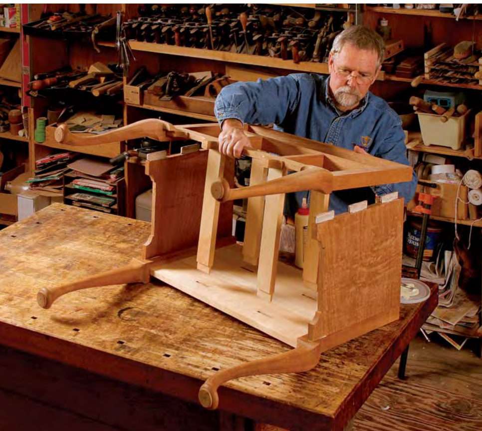
The final glue-up. Back and front assemblies are joined by gluing the side panels into the rear posts, gluing the interior kickers and runners into their mortises in the front, and then settling the front assembly into position.
