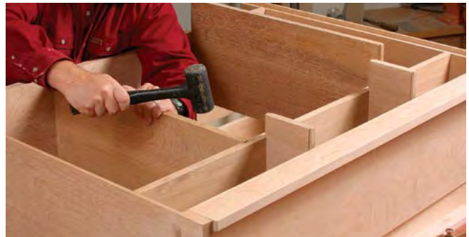
Long sliding dovetails with no binding. The trick is to slide in the dividers from the back almost all the way without glue, leaving about 2 in. exposed, and then apply glue to that exposed end and into the slot at the front. Now you can drive the divider home with a mallet.
