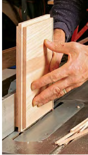
Cut tongues on the tablesaw. With the panels facedown, cut around the edges on all sides. Then ride the panel on edge and cut off the rest of the waste material, leaving the tongue. Keep the panel between the blade and the fence so the offcuts fall to the outside of the blade.
