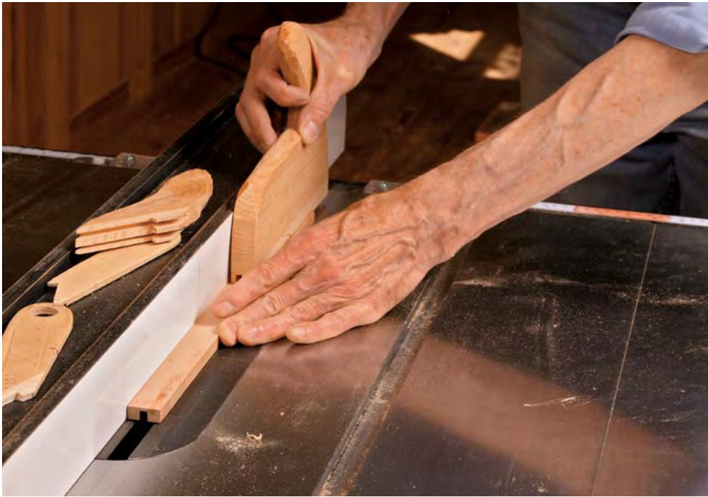
Make a groovy center strip. The center guide is simply a piece of wood with a groove that runs straight through.
