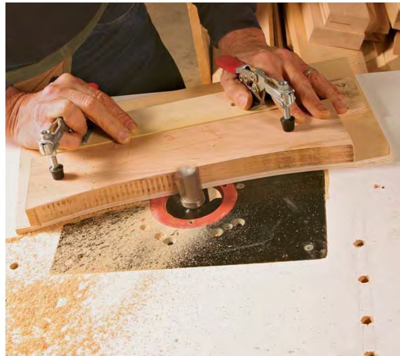
Cut the curve in the lower rails. Once the mortises are cut, the author bandsaws the curve of the lower rails close to the line and then template-routes the final curve.
