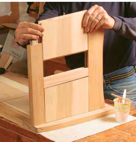
Glue up in stages: front and back first. The author uses Unibond 800 for more open time. Place the center panel into the bottom rail, add the dividers and then the end panels, set the top rail on, and add the legs last (left). Center marks help locate the dividers and keep everything evenly spaced. Angled cauls keep the clamps aligned. Next, the author uses a coping saw to cut the curve at the top of each leg and then uses a block plane to take it to its final shape (right).
