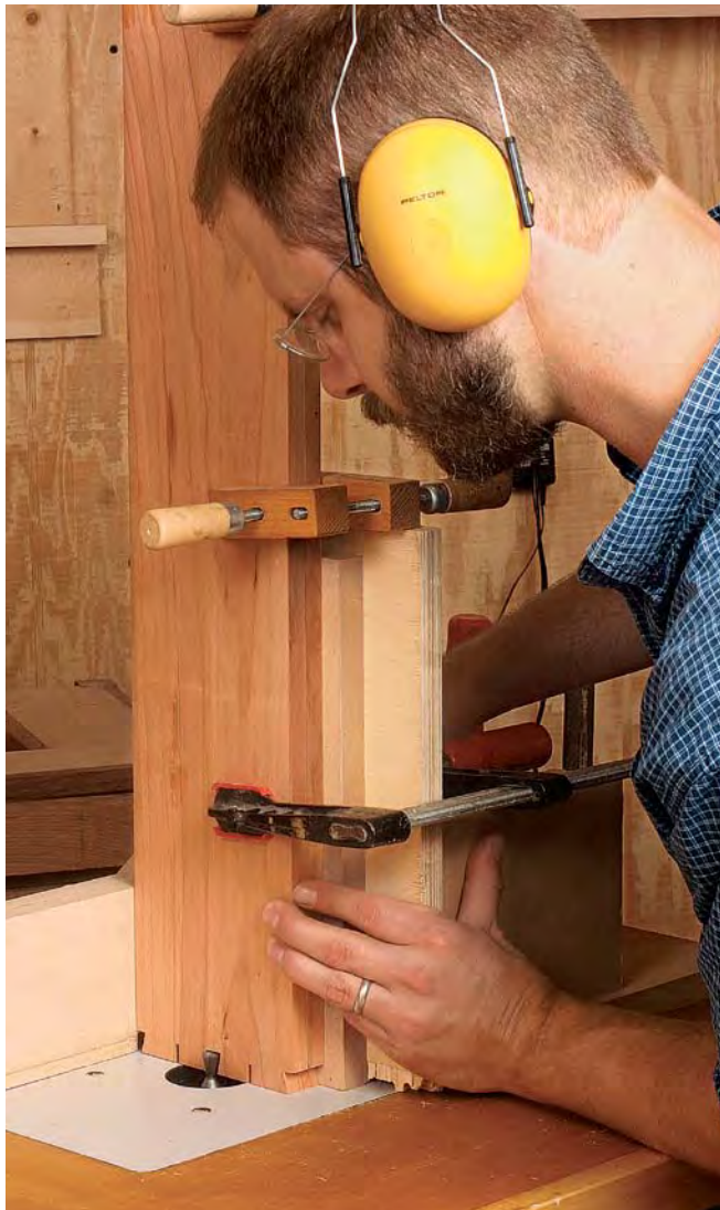
Cut the dovetails on the ends of the case sides. Using the router table equipped with a dovetail bit and a sled to support the stock, the author cuts the dovetails in short order.
