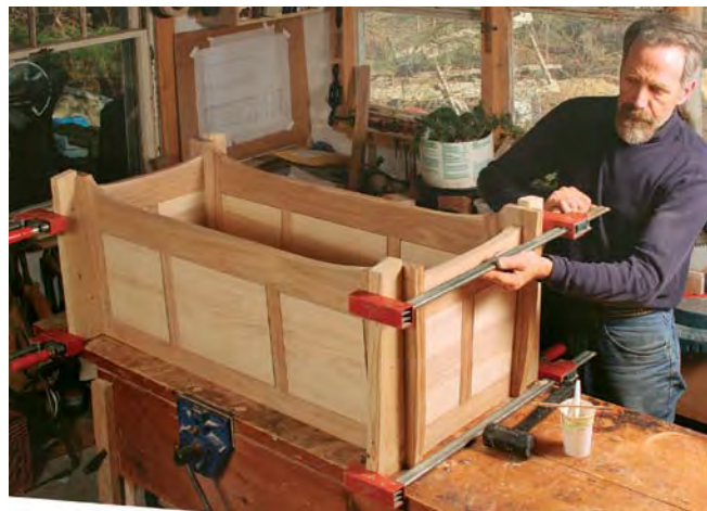
Glue up in stages: front and back first. The author uses Unibond 800 for more open time. Place the center panel into the bottom rail, add the dividers and then the end panels, set the top rail on, and add the legs last (left). Center marks help locate the dividers and keep everything evenly spaced. Angled cauls keep the clamps aligned. Next, the author uses a coping saw to cut the curve at the top of each leg and then uses a block plane to take it to its final shape (right).
