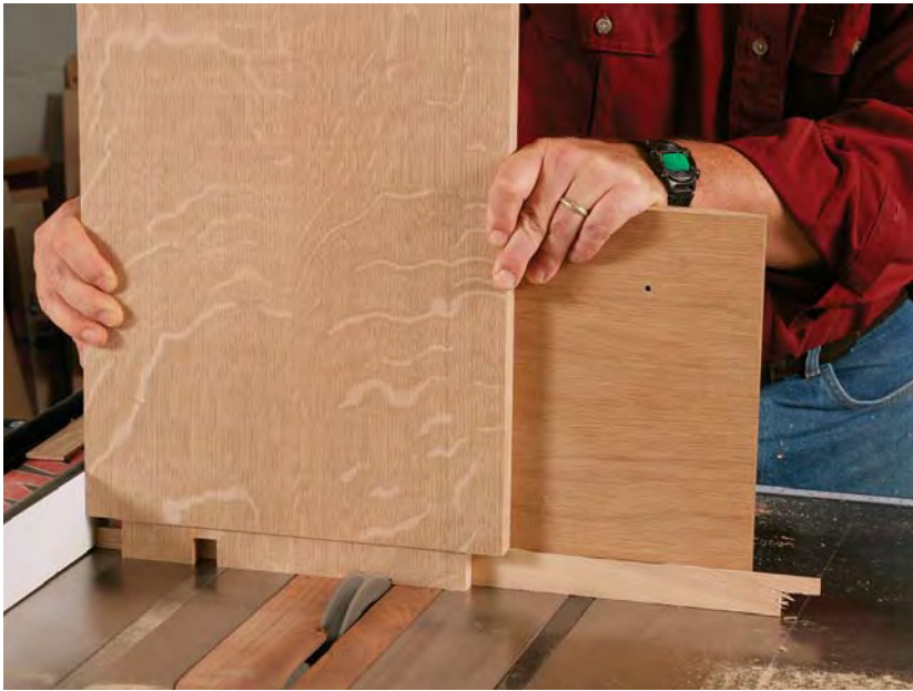
Two-part tenons. The dado blade does most of the work. After cutting the tenon cheeks and shoulders with a dado set, cut the through-tenons to width, using a tall fence to support the board. The scrapwood behind the tenons backs up the cut and reduces tearout.
