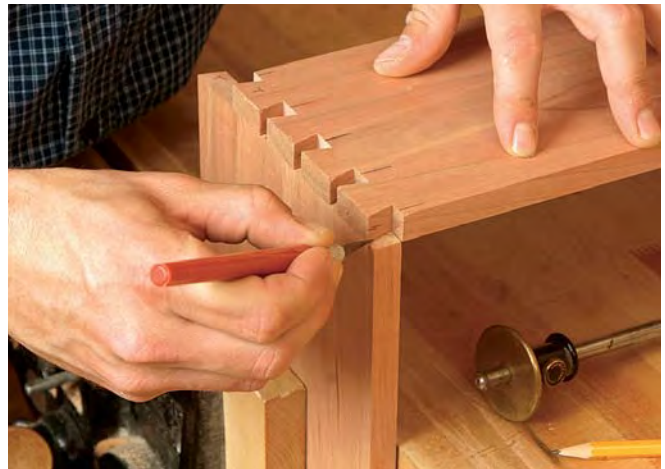
Mark the pins with the tails. Use a marking knife to scribe the pin lines on the ends of the top and bottom.
