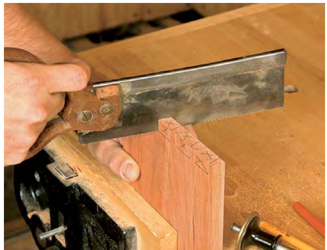
Hand saw the pin lines. With the knife lines as a reference, use a dovetail saw to cut along each pin line.
