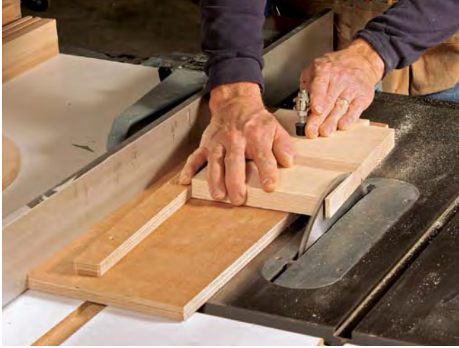
Make the panels. The side panels are tapered. To angle the outside edges, the author uses the same jig he used to cut the angle on the legs.
