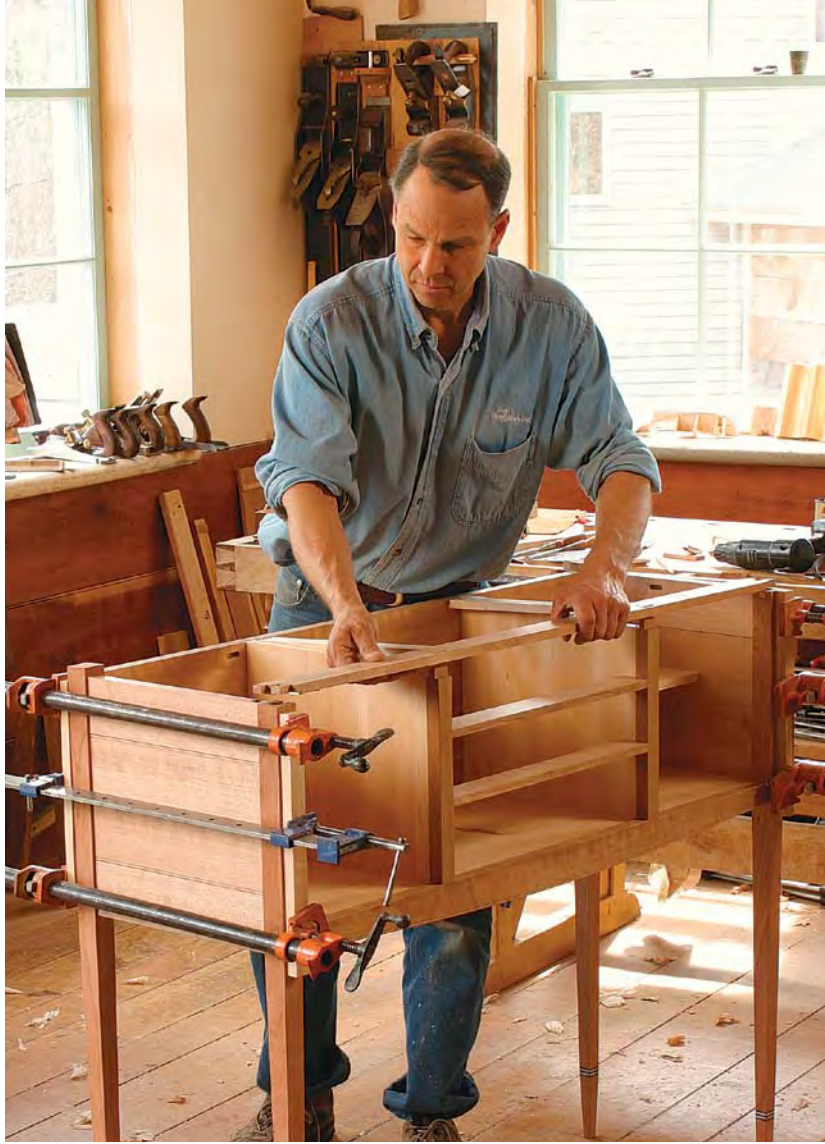
Add the top stretcher and kickers. With the case upright on the floor, install the stretcher. This is tricky because you have to glue in the kickers for the top drawer at the same time. The stiles of the drawer frame are tenoned into the stretcher. Drive wedges into the tenons, then screw the stretcher to the interior partitions.
