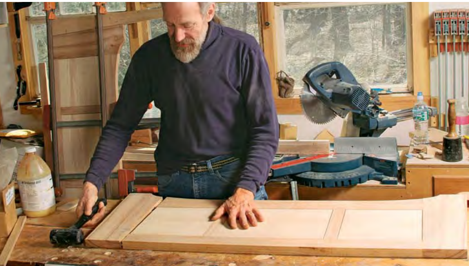
Glue up in stages: front and back first. The author uses Unibond 800 for more open time. Place the center panel into the bottom rail, add the dividers and then the end panels, set the top rail on, and add the legs last (left). Center marks help locate the dividers and keep everything evenly spaced. Angled cauls keep the clamps aligned. Next, the author uses a coping saw to cut the curve at the top of each leg and then uses a block plane to take it to its final shape (right).
