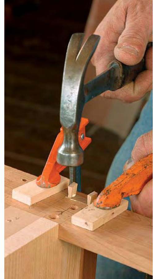
Add the top stretcher and kickers. With the case upright on the floor, install the stretcher. This is tricky because you have to glue in the kickers for the top drawer at the same time. The stiles of the drawer frame are tenoned into the stretcher. Drive wedges into the tenons, then screw the stretcher to the interior partitions.
