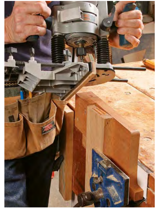
Mortise and shape the rails. End rails have angled shoulders. The author cuts the 3° angle on one end of the rail and then uses a full-size drawing to mark the length (left) of the other end. He uses a simple vise-mounted jig when mortising the ends. It holds the rails square and gives a surface for the edge guide to ride on. The jig works for the angled rails too (right).
