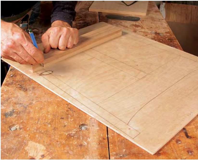
Mortise and shape the rails. End rails have angled shoulders. The author cuts the 3° angle on one end of the rail and then uses a full-size drawing to mark the length (left) of the other end. He uses a simple vise-mounted jig when mortising the ends. It holds the rails square and gives a surface for the edge guide to ride on. The jig works for the angled rails too (right).
