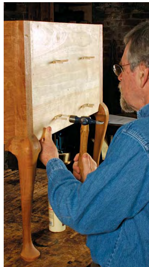
Wedge the tenons. The center runners are secured in back with wedged through-tenons. Glue the wedges and tap them home. When dry, saw them off and plane them flush.
