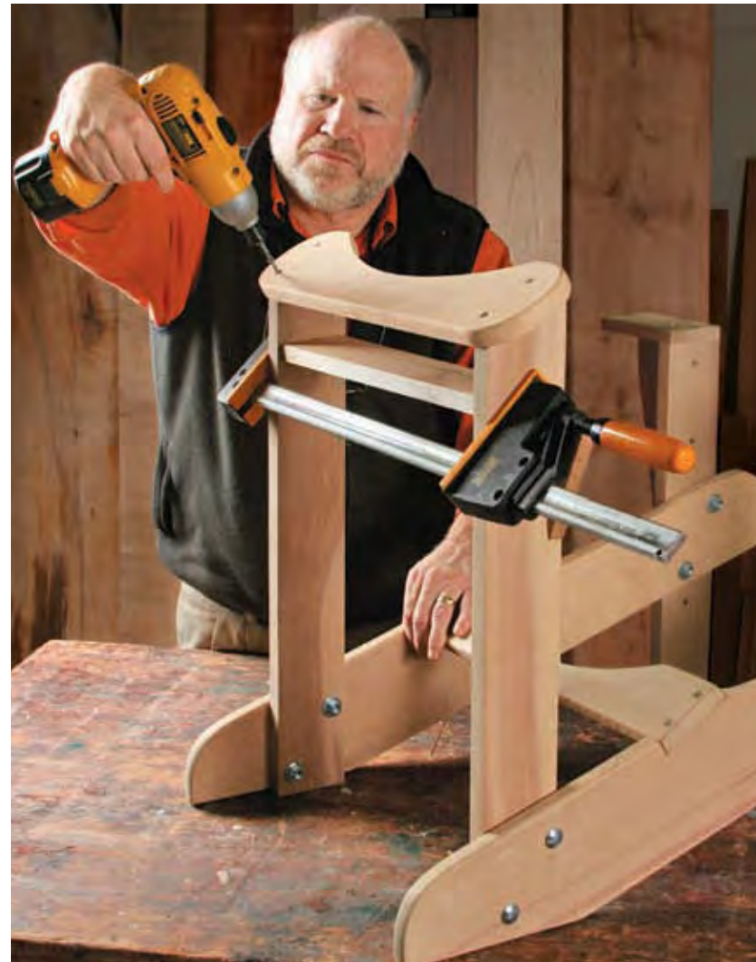
Attach the upper cradle. Use a temporary spacer board to ensure that the risers stay parallel when the upper cradle is attached.
