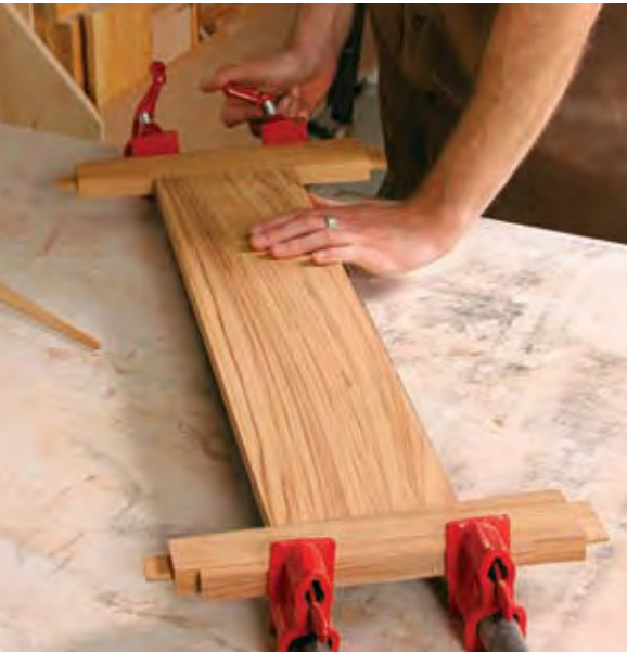
Glue the center rail to the center back splats. Jensen uses the cutoff pieces from the tapering process to create a square clamping surface (above). The tapered back splats, center rail, and crest rail complete the glue-up (right).
