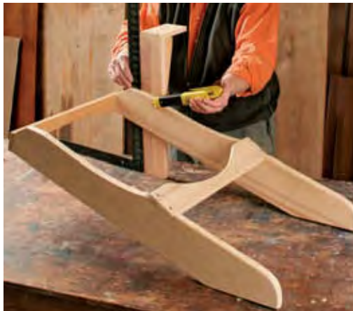
Make a subassembly. Screw the stretcher to the front and follow with the lower cradle.
