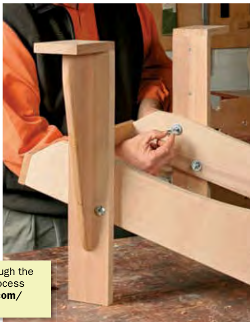
Attach the upper cradle. Use a temporary spacer board to ensure that the risers stay parallel when the upper cradle is attached.
