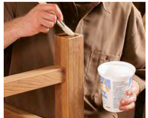
Seal the legs. Seal the bottoms of the legs by coating them with the same epoxy used in the glue-up.
