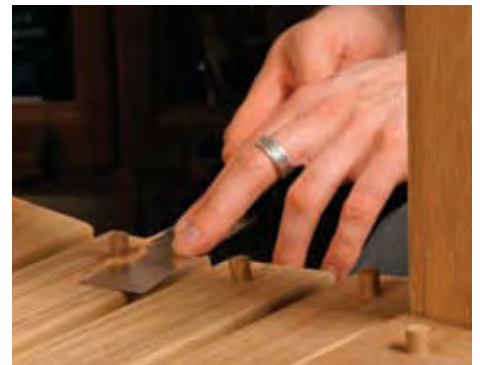
Plug the screw holes. After screwing the seat slats down, glue in plugs, then cut them flush.
