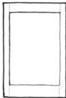
Restate the shape Keeping the design as simple as possible preserves the essential shape of the opening.
