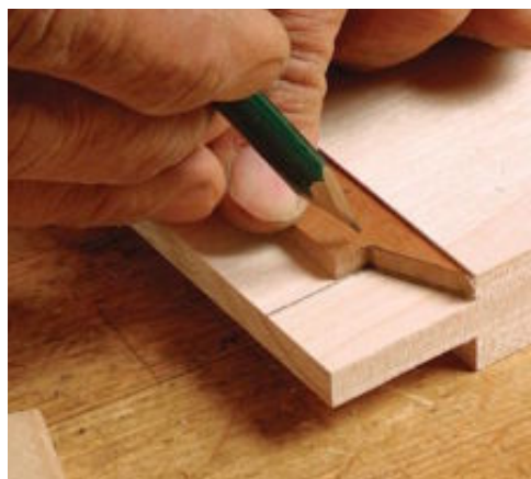
Template simplifies layout. Mark out the angled haunch on the tenon using a template.
