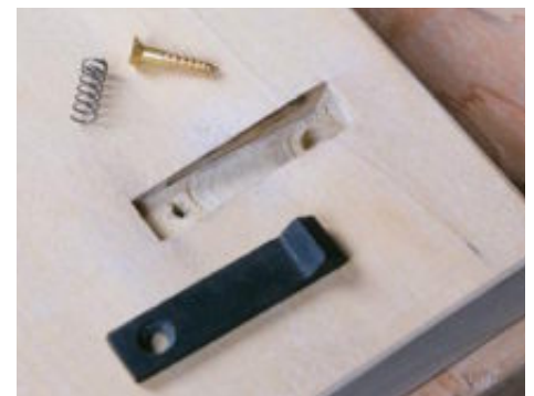
Catch assembly. The spring sits in a hole bored in the deep end of the mortise, and the screw threads through the back end of the flipper.
