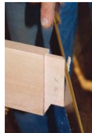
Handwork is fast and accurate enough. A dovetail saw makes quick work of trimming the angled haunch and mitering the ends of the tenons.
