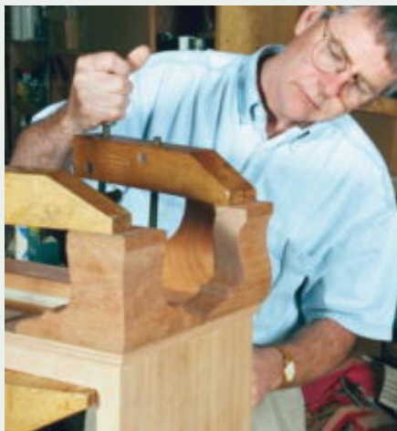
Attach the feet. Miter each section and glue the halves to each other, then the whole foot to the bottom of the case. Add glue blocks as reinforcement.
