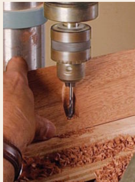
Pocket-hole jig. Construct a small jig to hold the apron at approximately 10^\circ while drilling pocket holes with a Forstner bit.
