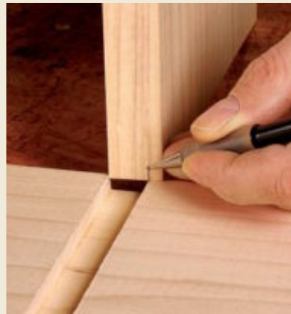
Mark and cut the rabbet. First, mark the rabbet location on the end of the shelf (left), then use a bearing-guided rabbeting bit to cut the rabbet (above).
