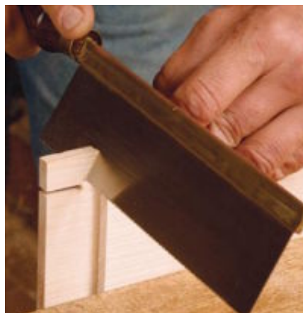
Handwork is fast and accurate enough. A dovetail saw makes quick work of trimming the angled haunch and mitering the ends of the tenons.
