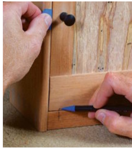
With the case assembled, transfer the mortise location. Use a piece of tape to hold the door flush with the outer edge of the case.
