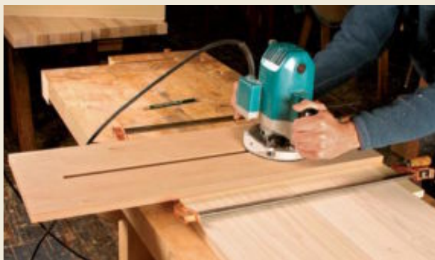
Rabbeted dado starts with a dado. A T-square jig helps cut a dado across the side. The slot in the jig is just wide enough to accept the bearing of a top-mounted bearing-guided straight bit.
