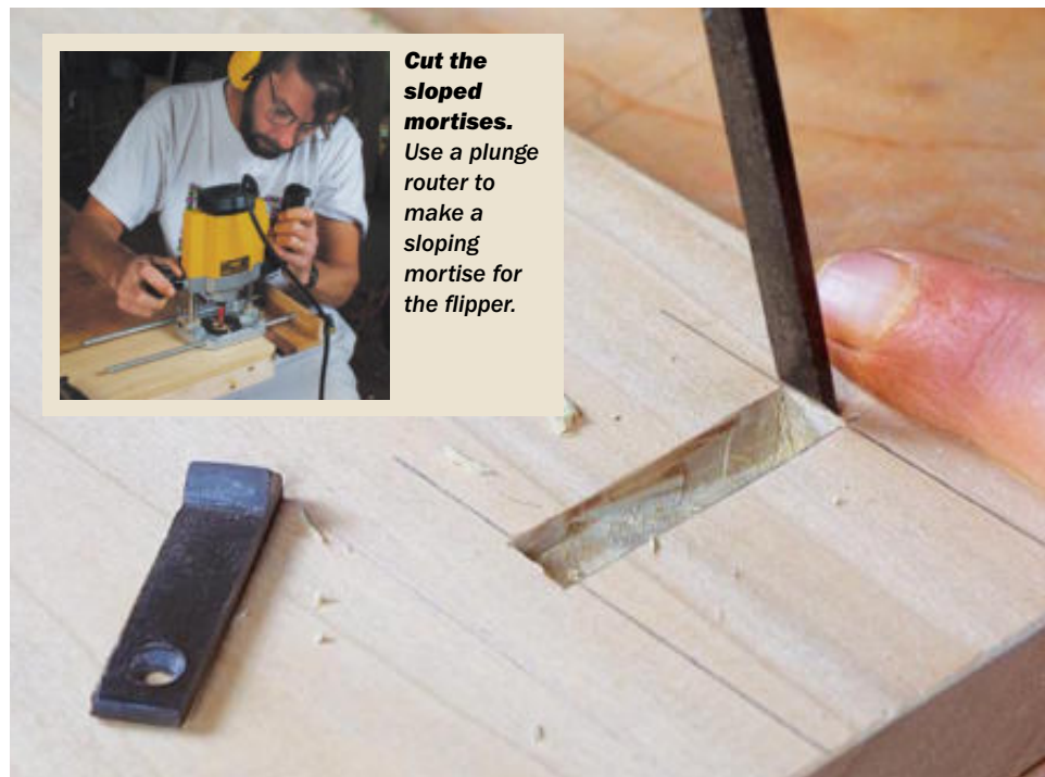
Chisel the mortise to length. Scribe the length and width, then pare close to the layout lines. Check the fit often as you work; you don't want to make the mortise too wide.
