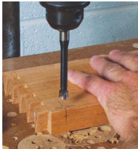
Drill mortises before gluing up the case. One set of magnets is recessed into mortises drilled into both the case top and bottom.
