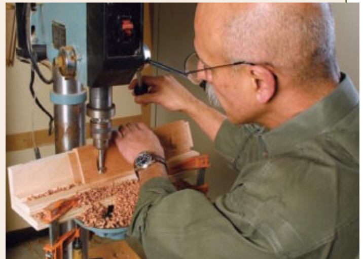
Pocket-hole jig. Construct a small jig to hold the apron at approximately 10^\circ while drilling pocket holes with a Forstner bit.
