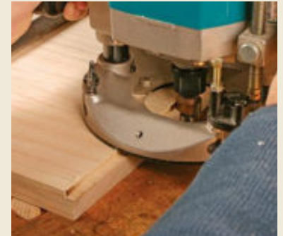
Mark and cut the rabbet. First, mark the rabbet location on the end of the shelf (left), then use a bearing-guided rabbeting bit to cut the rabbet (above).
