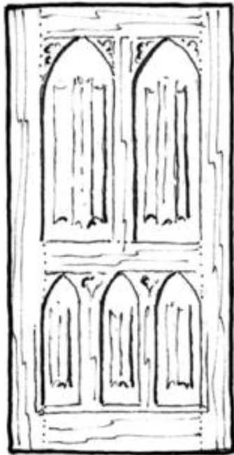
Victorian Gothic Emphasis on vertical elements, pointed arch panels, linen-fold carving; multicolor finishes on walnut or fumed oak.
