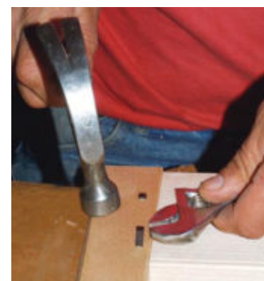
Pins are an insurance policy. Small hardwood pins will hold the joint tightly, even if the glue fails. Hack leaves the outside end of the pin square and holds it with a wrench as he hammers it home.
