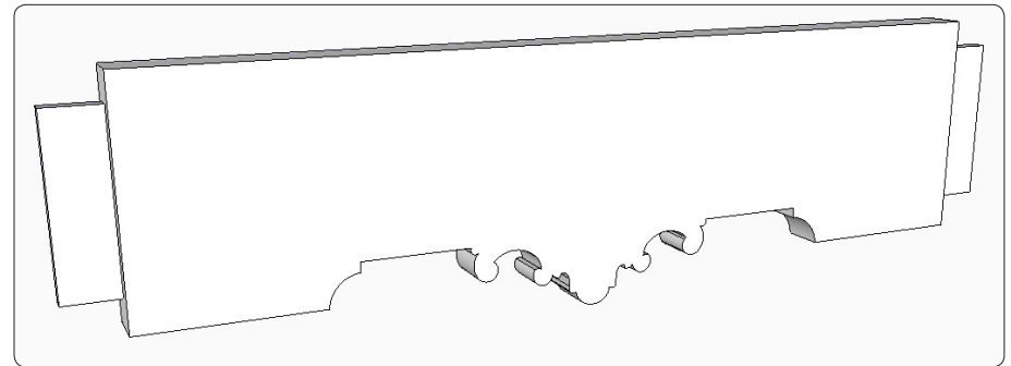
Figure 25. Lengthening an elaborate component like this side skirt means working at the ends and leaving the middle alone.
