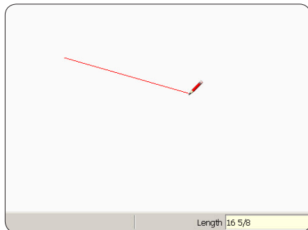
Figure 4. To draw a line to an exact length, type the length. The number appears in the Measurements Box.
