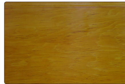
Figure 10. Photograph an existing piece that duplicates or closely matches the texture and finish you want. This photo shows the seedlac finish I used on the blanket chest.
