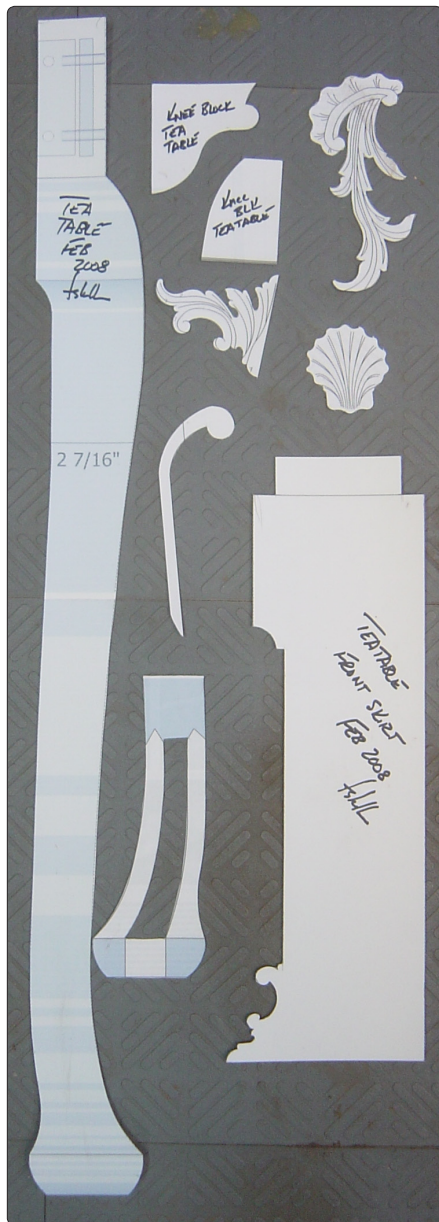
Figure 2. Templates for the legs and carvings on a tea table.
