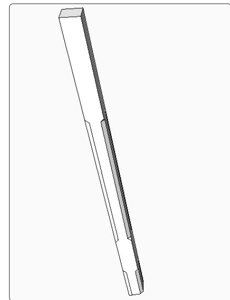
Figure 13. Delete waste lines to complete the chamfers.
