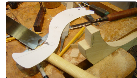
Figure 6. The hidden joinery on the template lets me mark accurate cutting locations.
