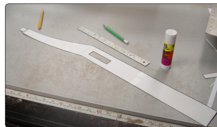
Figure 4. To make a template, I piece together the printouts, paste the result onto poster board, and then carefully trim it.
