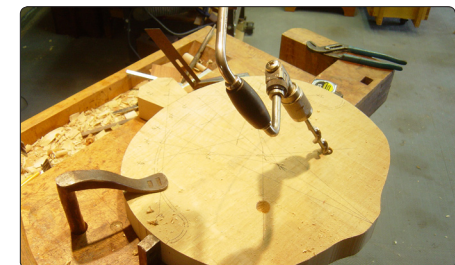
Figure 7. Sight lines transferred from the template to the seat help me drill the sockets at the correct angles.
