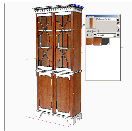
Figure 22. Apply the vertical-grain texture to all the appropriate faces, then do the same for the horizontal-grain faces.
