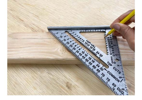
**Tip** – Be sure to use a sharp pencil (not a carpenter's pencil) for this. Many speed squares feature a sawtooth along the <u>ruler</u> edge which is very helpful.
