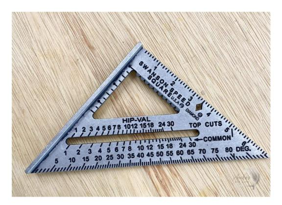
A <u>Speed Square</u> or <u>carpenter's square</u> is one of the most basic and essential tools in woodworking. It is extremely inexpensive, accurate, and has a wide variety of uses!
