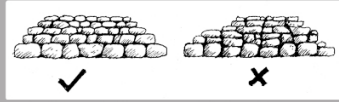
Correct coursing of joints on the left. Incorrect on the right, resulting in many running joints.
