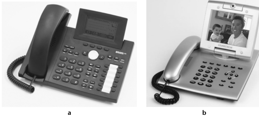
Figure 2.6 Desktop SIP phones: (a) Business SIP phone; (b) Consumer SIP videophone (a) Courtesy: snom Technology; AG (b) Courtesy Grandstream Networks, Inc.
