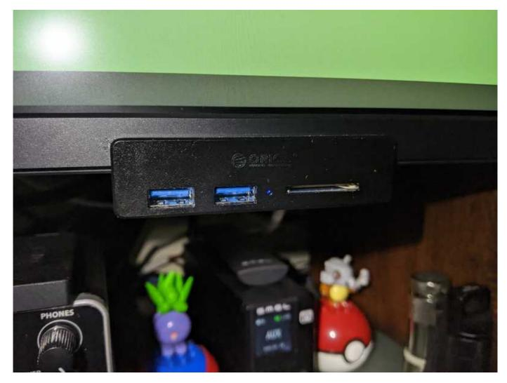
I think for most of us, we have the front IO on our case for easy usb access and what not. In this instance, that's where the Orico MHP4U that I mentioned above comes in. This allows you to plug devices into either OS at any point of time and the fact that they are sitting below the screen of the OS should be an easy
