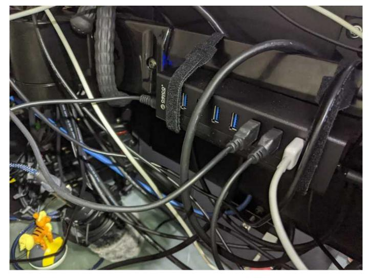
The GoPro is configured to output the live view through HDMI and is powered via the Orico 7-Port USB Hub. This hub has no other use than to provide power for the components. The output of the GoPro goes to the HDMI splitter and, the splitter is connected to each of the USB hdmi capture dongles. This allows us to have real time video input for both MacOS and Windows.
