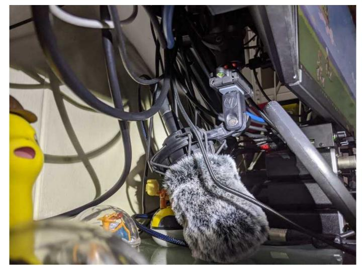
The microphone set-up involves mounting the microphone to the Ulanzi MT-11 tripod and hanging it upside down from my monitor mount, so it's basically hanging at the bottom. Placed a simple fur cover that takes care of wind (from my fan) and a pop filter hovering on top of it.
