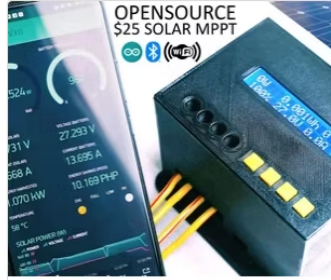
1kW Arduino MPPT Solar Charge Controller (ESP32 + WiFi) by ASCAS in Arduino
