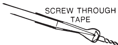
Fig. 5-15. One way to hold a screw before starting it is to tape it to the screwdriver blade; use tape that will break easily once the screw is started.
