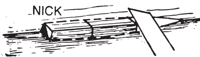
Fig. 9-3. If a long cut will stop before the end is reached, cut a nick at its end first, and slice the waste part into several pieces.
