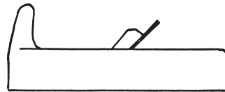
Fig. 2-16. This plane, with a horn-shaped handle in front, is pulled rather than pushed.
