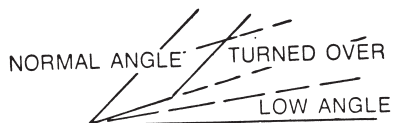
Fig. 2-17. A single iron, turned over, can produce the same cut as one normally situated and used with a cap iron.
