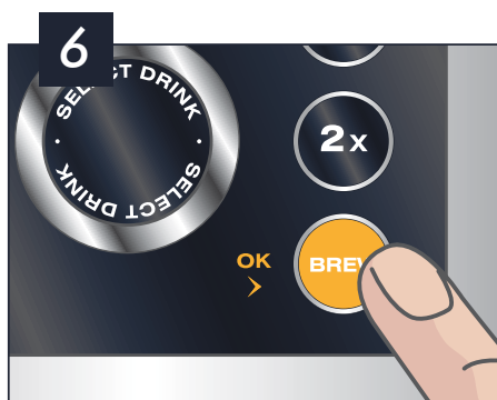
6 Press OK Button. The machine will prime. A little water will be released by the hot water spout. The machine will then switch it off automatically.
